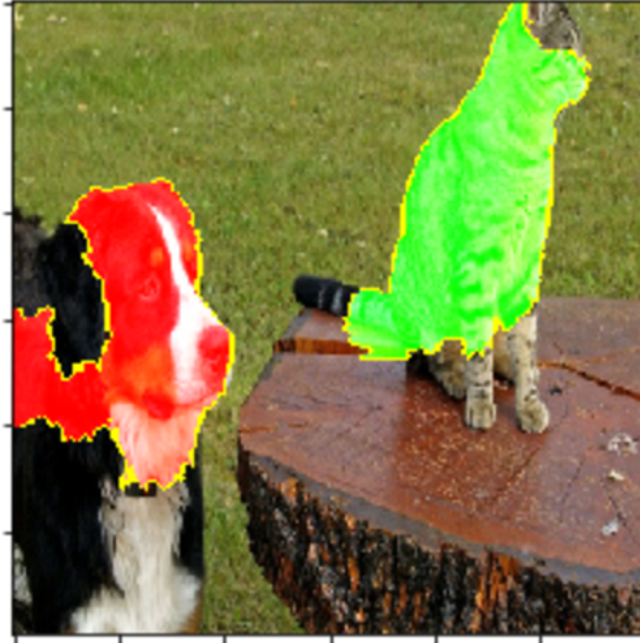
Figure 2.9: With green color those areas are highlighted which supported the "Cat" prediction, conversely the red ones didnt. Source: https://github.com/marcotcr/lime
