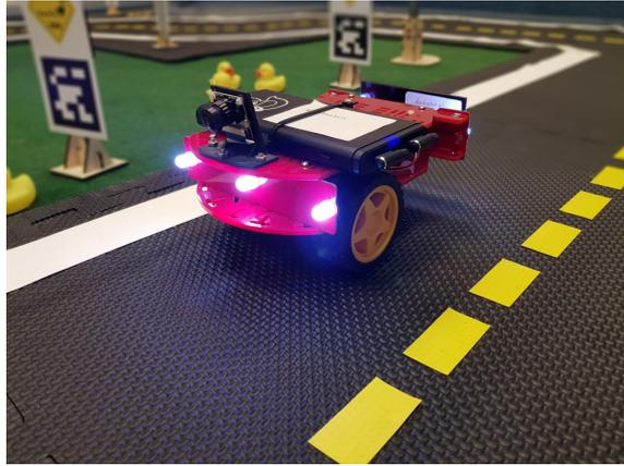
**Figure 4.2:** Duckiebots are small three-wheeled robots with a forward-facing camera. It has to be controlled by processing the camera images and giving wheel speed commands.
