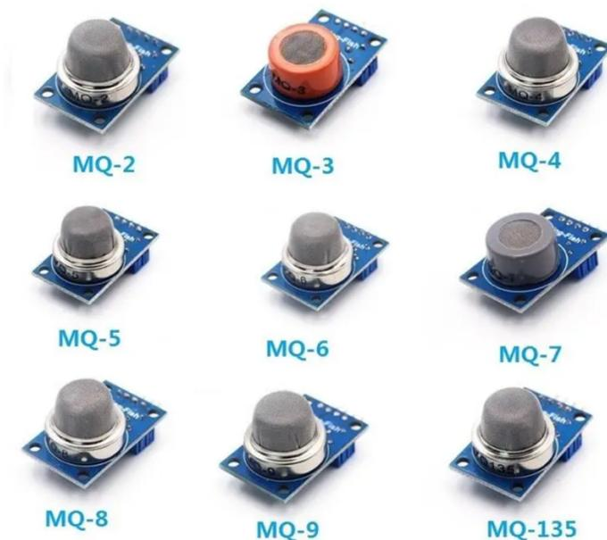
Figure 3.2 MOx Sensors Embedded in E-Nose Device<sup>2</sup>
