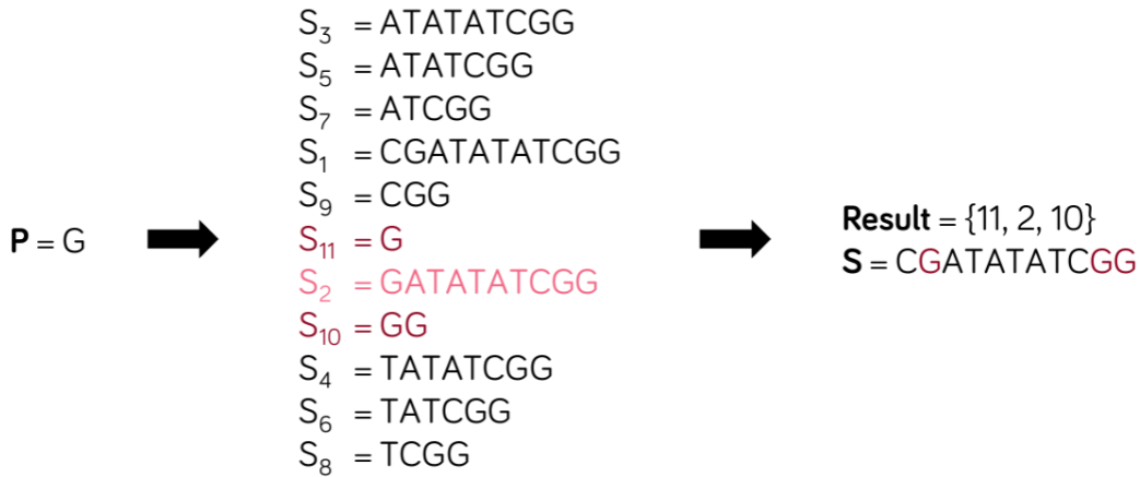
Figure 2: Example of suffix array based pattern matching for S = CGATATATCGG and P = G .
