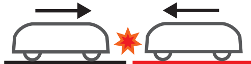
Figure 5.15 Unsafe configuration. If a train comes in the opposing direction, they will crash.
