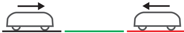
Figure 5.14 Safe configuration. The train from the failed group can be stopped on the buffer rail.
