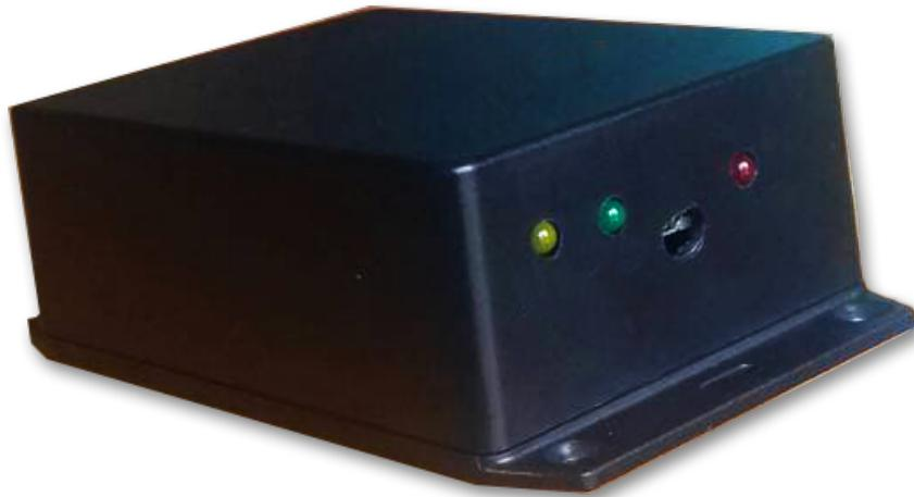
**Figure 3.1:** *The plastic case that stores the hardware: the RFID-enabled, UWB based, automated, wireless tracking module*
