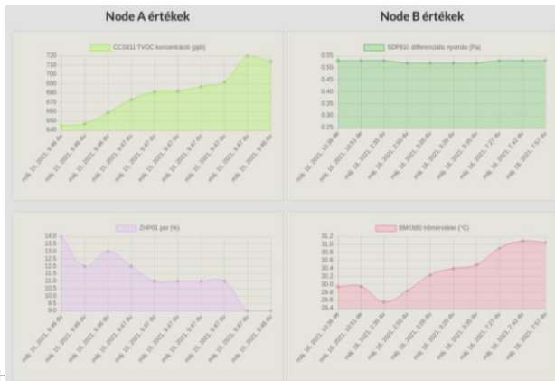
Fig. 9. Recorded data visualization of two nodes (Node A – on the left, with TVOC measurement and particle count in the ambiance; Node B – on the right with differential pressure measured inside a reflow oven and a temperature increase in the ambiance of the oven.)
