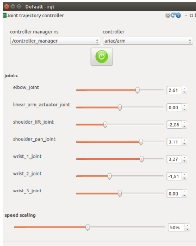
Figure 5.3: This is the graphical user interface for executing joint-space trajectories on a group of joints
