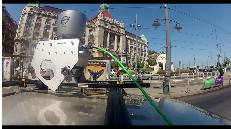
Figure 2.2: Velodyne HDL-64E sensor on the streets of Budapest (pictured in front of Gellért Bath)
