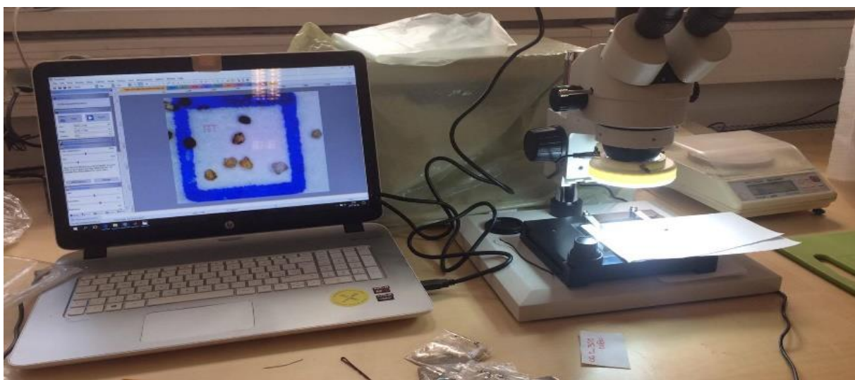
Fig.1.2. Taking pictures of the grains with a camera attached to a microscope in the Laboratory of the Department of Mechanics, Materials and Structure, Budapest
