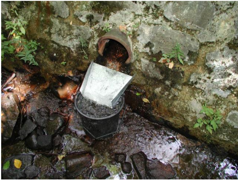
Figure 7. Volumetric discharge measurements method [source: http://www.state.nj.us/dep/wms/shvanda_stream_gaging.pdf ]
