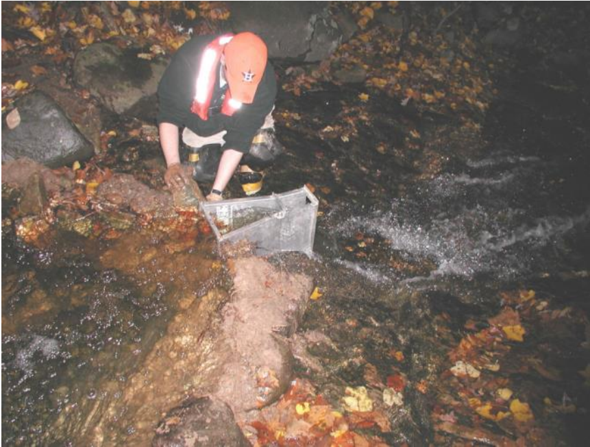
Figure 8. Discharge measurement with a portable Parshall Flume [source: http://www.state.nj.us/dep/wms/shvanda_stream_gaging.pdf ]
