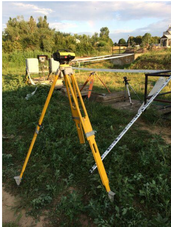
Figure 20. Leica digital leveling instrument
