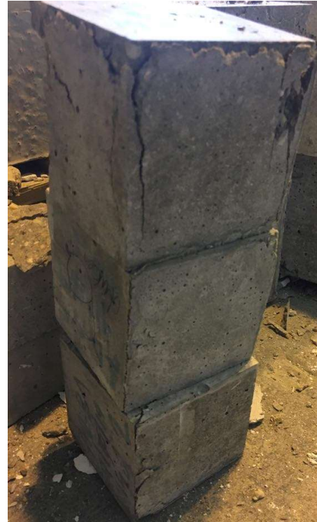
b) Cube specimen with edge length of 100 mm
