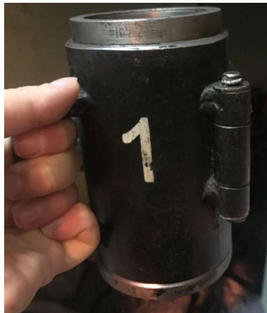
a) Cylinder mold with dimensions of 60x120 mm
