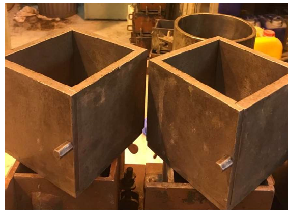
b) Cube mold with 100 mm edge length
