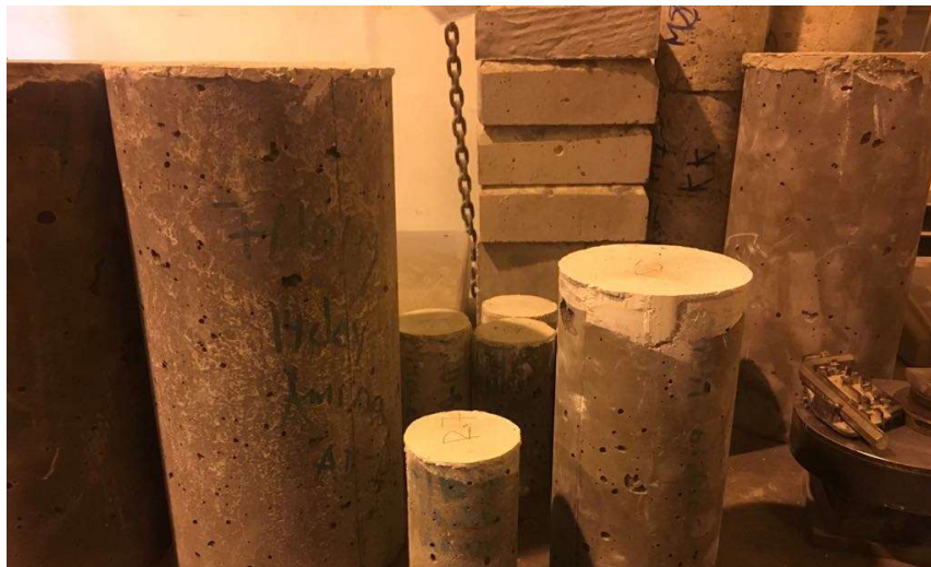
Figure 14 Capped cylinder specimens with different sizes
