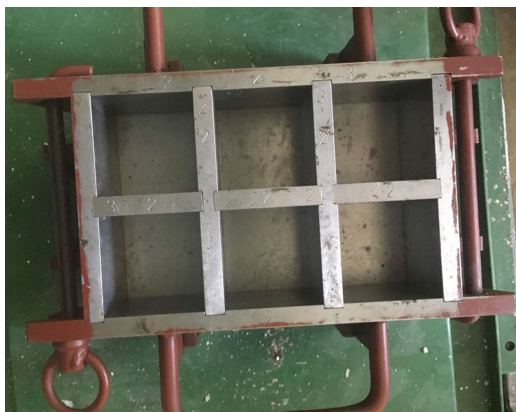
a) Cube mold with 50 mm edge length
