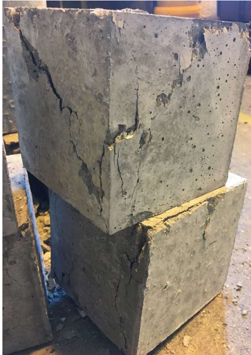
a) Cube specimen with edge length of 150 mm
