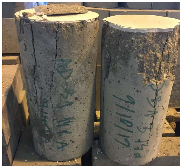
c) Cylinder specimen with dimensions 150x300 mm
