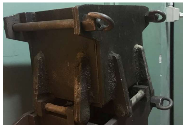
d) Cube mold with 200 mm edge length
