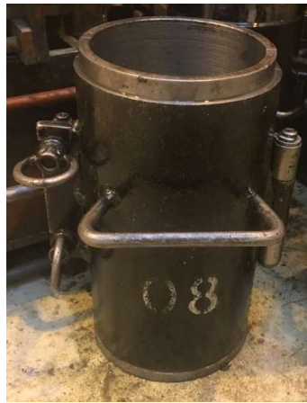
b) Cylinder mold with dimensions of 100x200 mm
