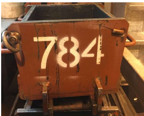
c) Cube mold with 150 mm edge length
