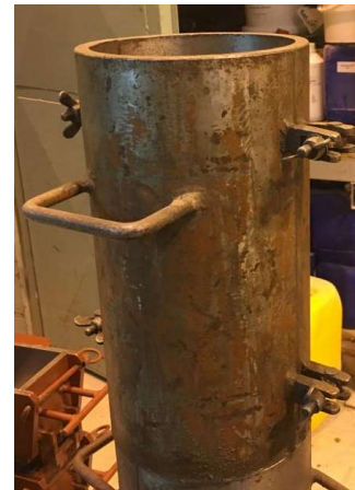
c) Cylinder mold with dimensions of 150x300 mm
