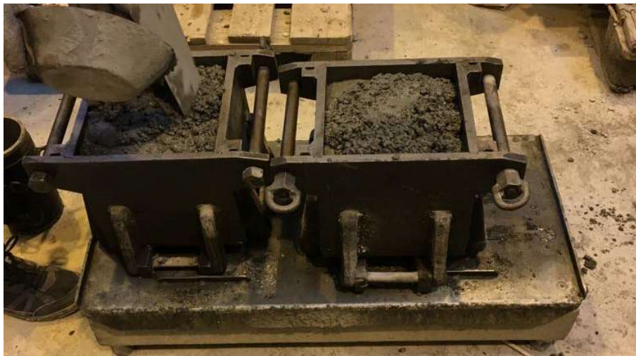
Figure 13 Casting concrete on a vibrating table
