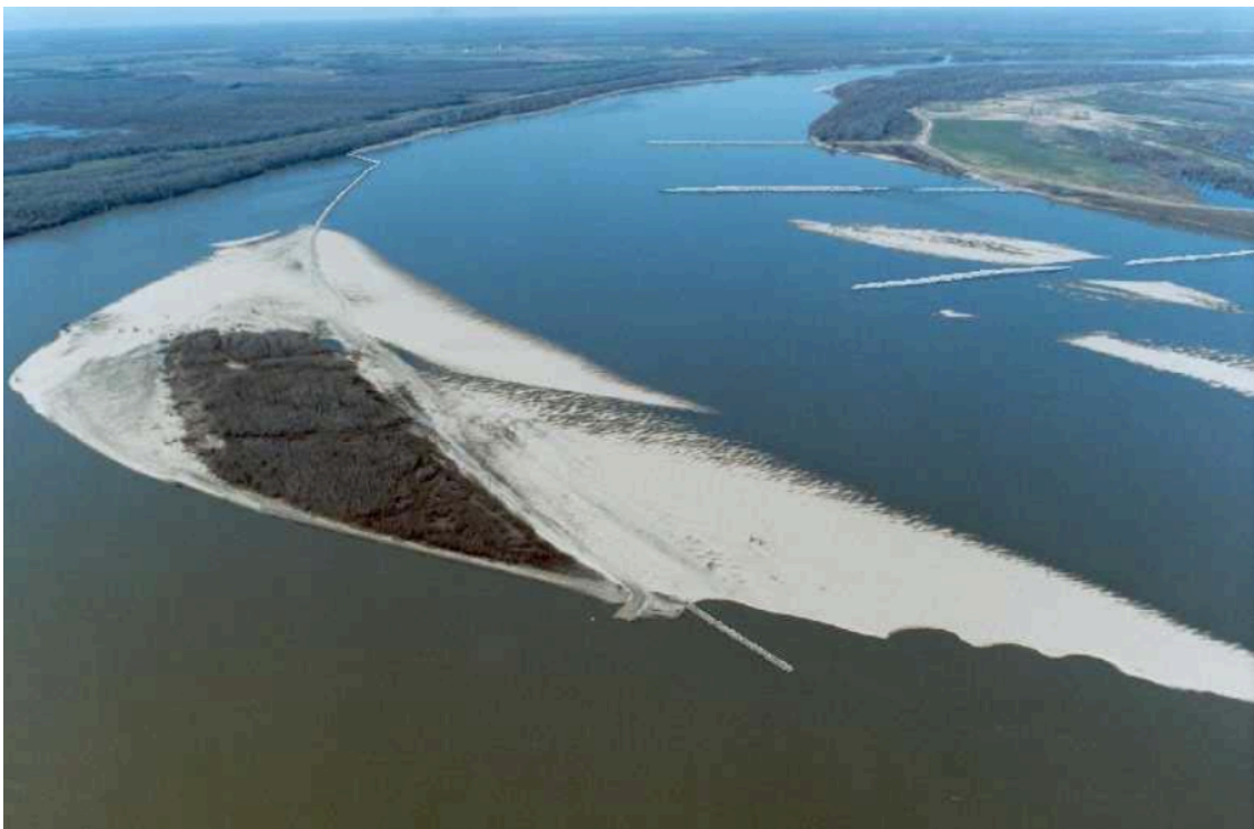
Fig. 47.: Dredging and revetments at Choctaw bar of the Mississippi River to improve navigation. [17]
