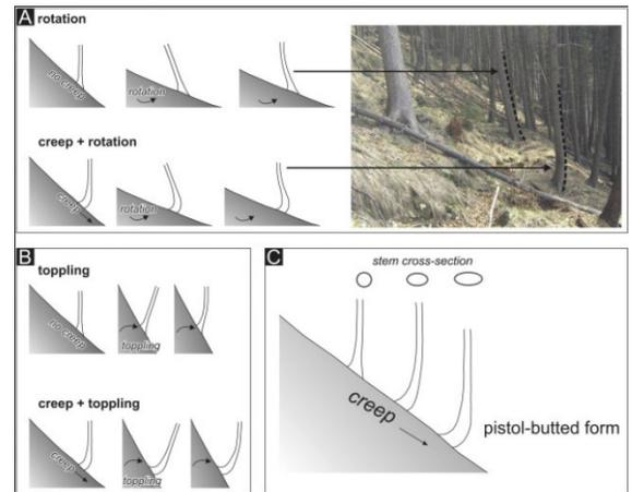
Figure.58(Tree deformation as an indication to slope movement) [28]
