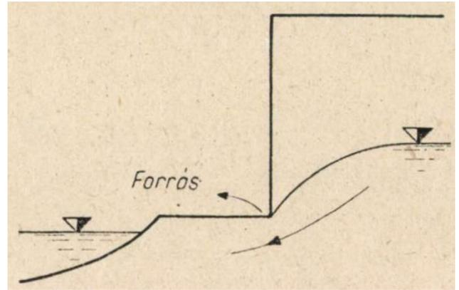
Figure.7 (Hydrogeological conditions under high cliffs) [25]
