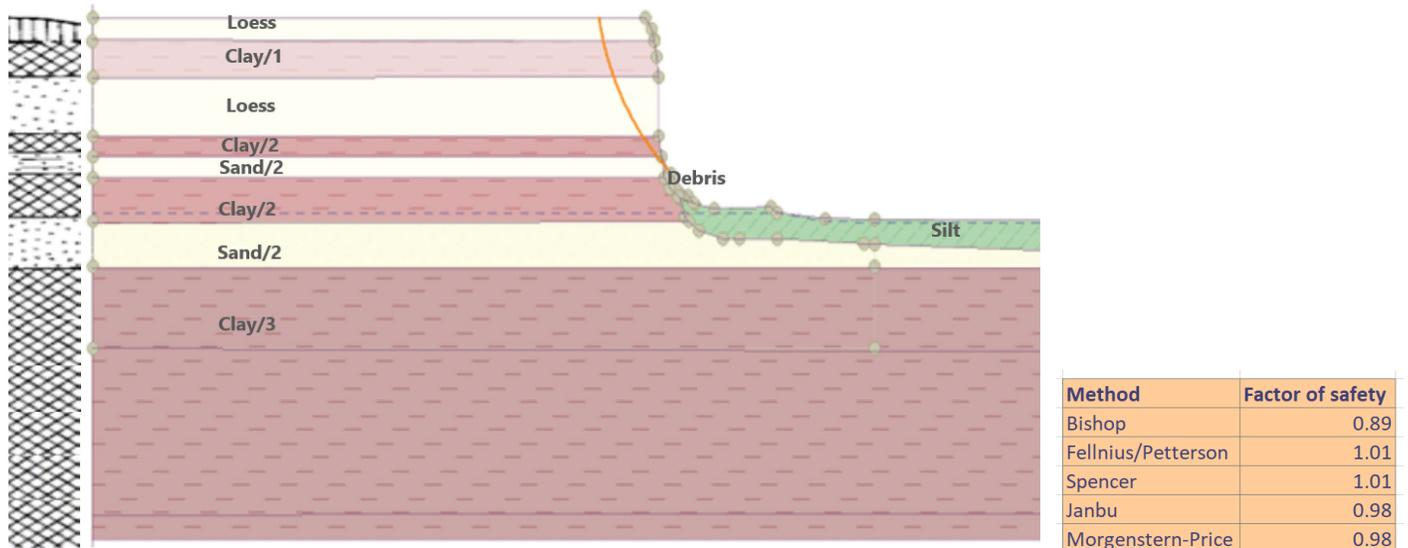
The image showing the modeled slope is shown above, along with the model we can see the literature layer order that was used for modeling. The slip surface that was identified by the limit equilibrium methods implemented can be seen.
