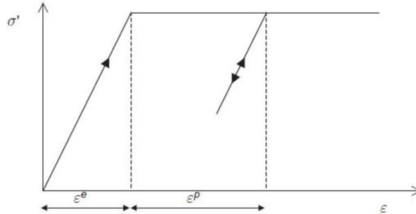
Figure.42 (Elastoplastic material model) [23]
