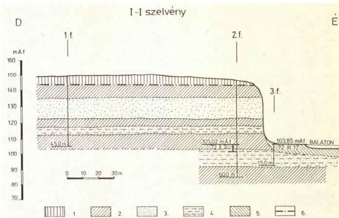
Figure.17 (Balatonföldvár High Cliff Section) [4]
