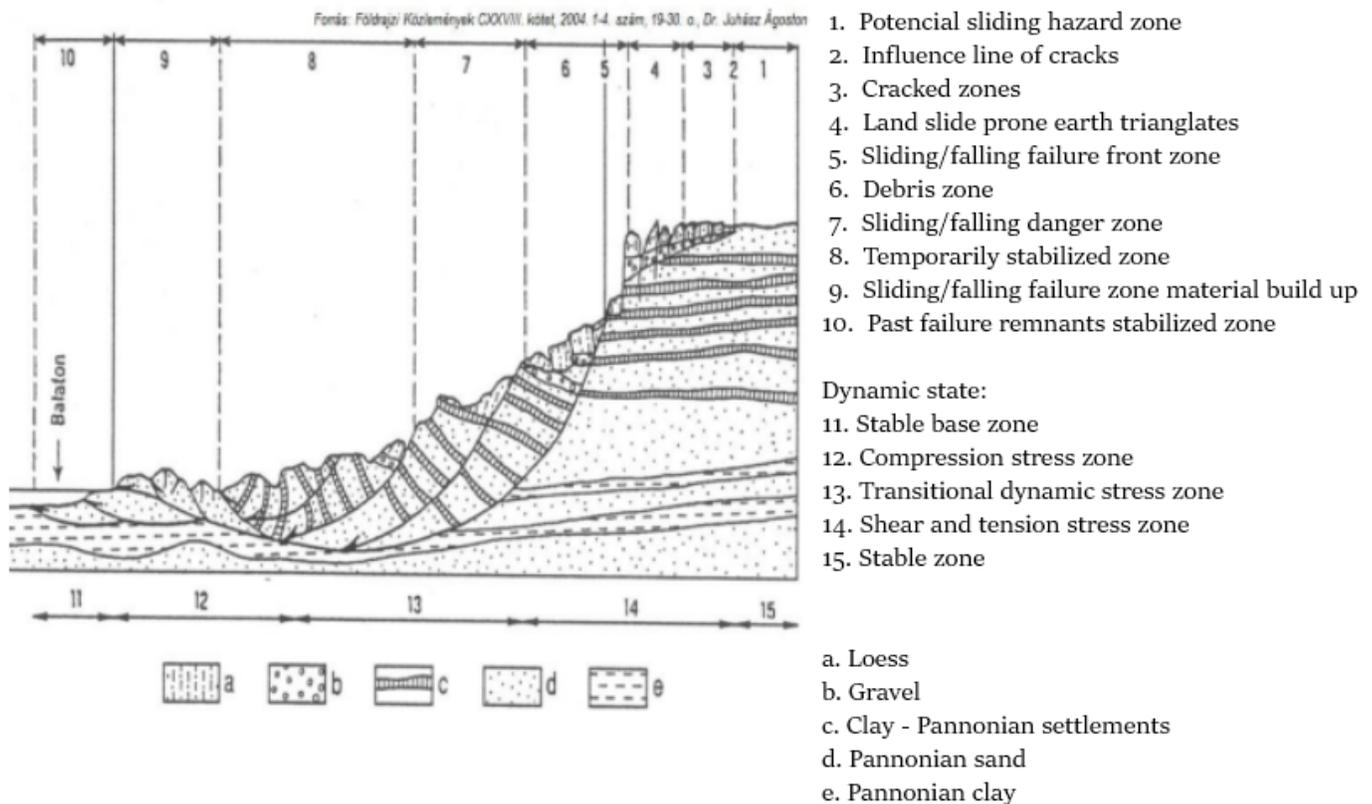
Figure.28 (Geomorphological model of slumps)[7]
