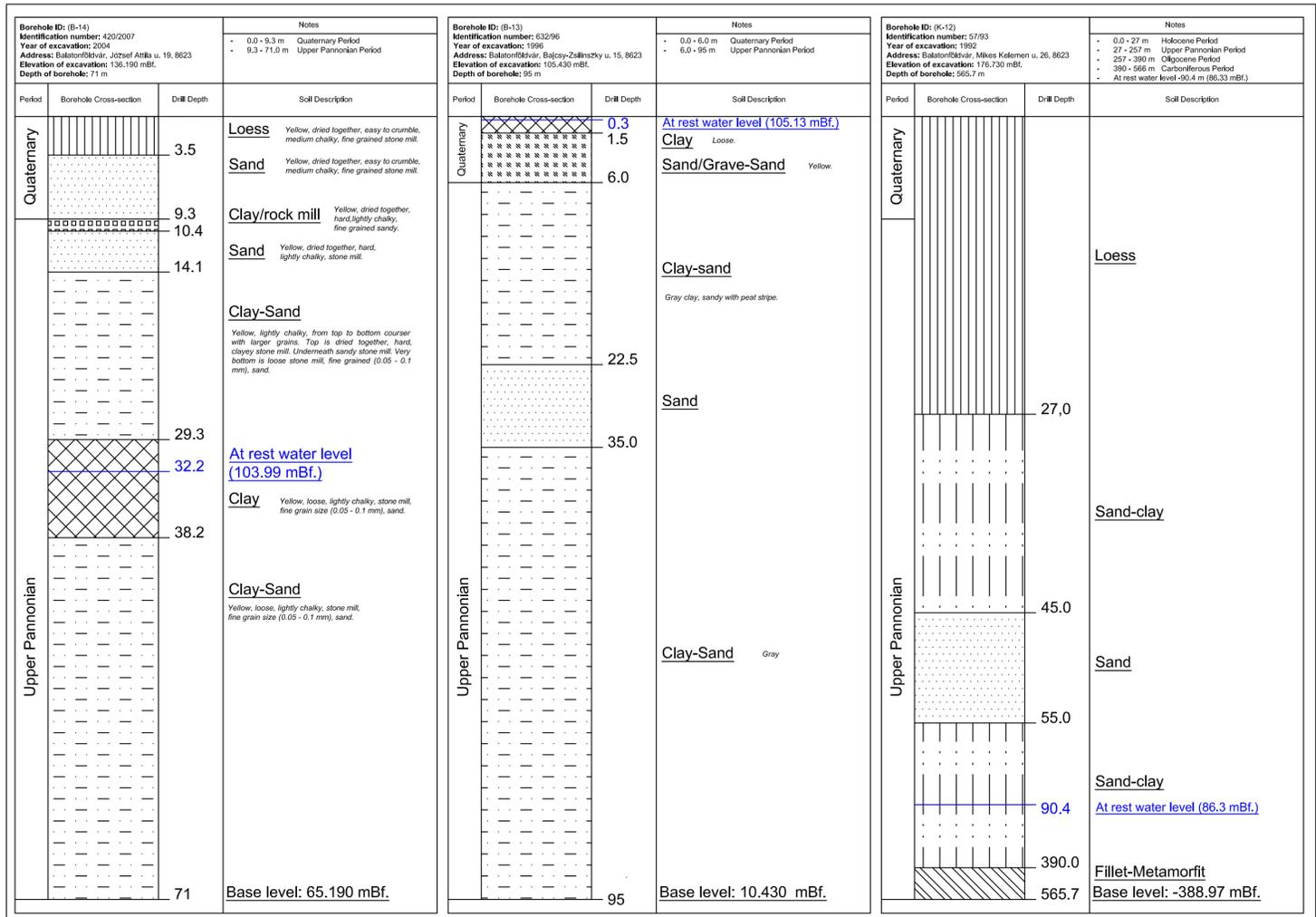
Figure.50 (Borehole cross sections ( B14, B13, K12))
