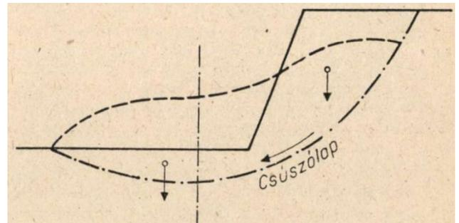
Figure.9 (Slope failure force balance) [25]
