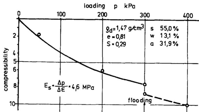
Figure.37 (Compressibility and Elastic Modulus of Loess) [13]
