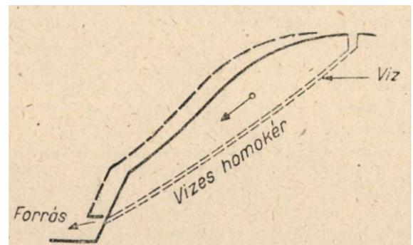
Figure.3 (Real sliding failure sliding plane) [25]
