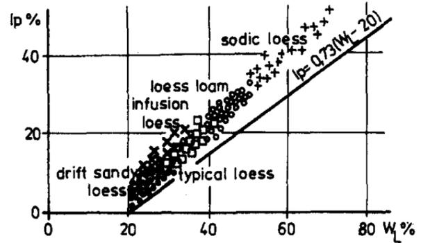
Figure. 35 (Plasticity and grain size of loess types) [13]
