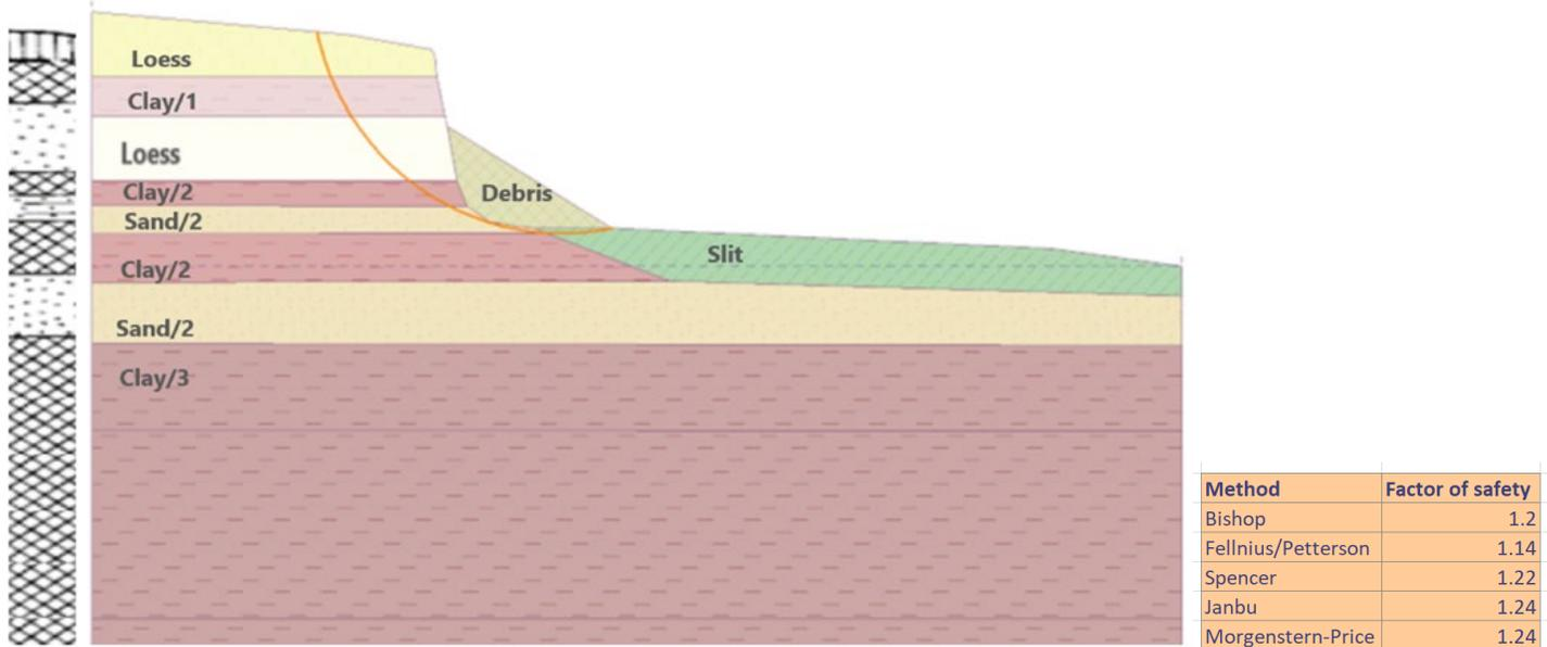
The critical condition no longer appeared as a local failure at the edge of the cliff but as a global failure within the sand layer. Applying the optimization check for all within an all-encompassing slip surface, the factor of safety failed the required safety factor of 1.35 according to MSZ EN 1997 (Eurocode 7).
