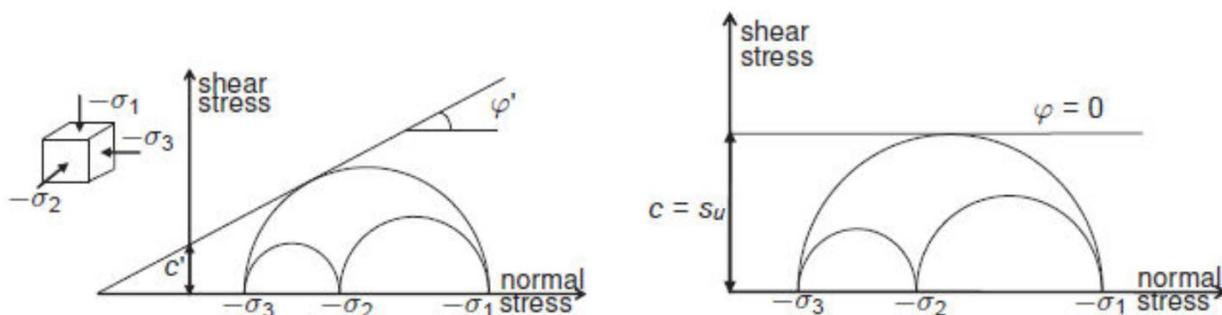
Figure.43 (Drained and Un-drained Mohr-Coulomb failure envelope curves) [23]
