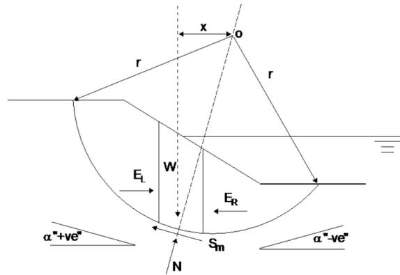
Figure.40 (Forces associated with Bishop method of slices) [21]
