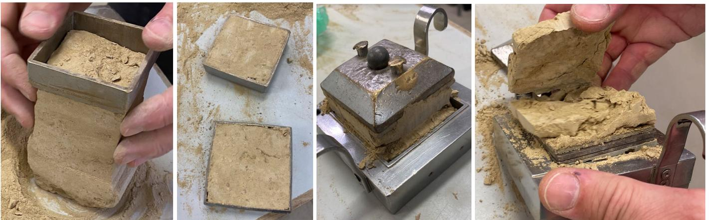
Figure.46 (Shear-box test)
