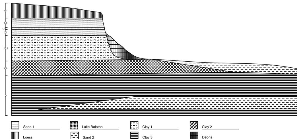
Figure.51 (Cross section created from borehole cross sections ( B14, B13, K12))
