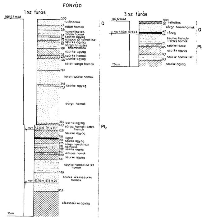
Figure.24 (Fonyód borehole section) [5]
