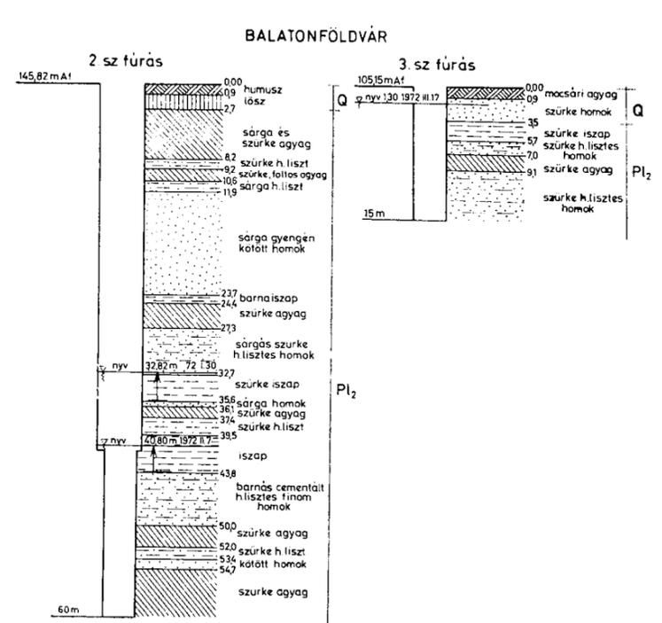
Figure.25 (Balatonföldvár borehole section) [5]
