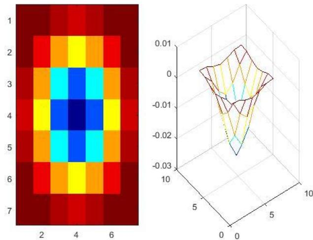
**Figure 12.** Parameter of the Gaussian filter: blob (tennis ball) size = 7 pixel diameter
