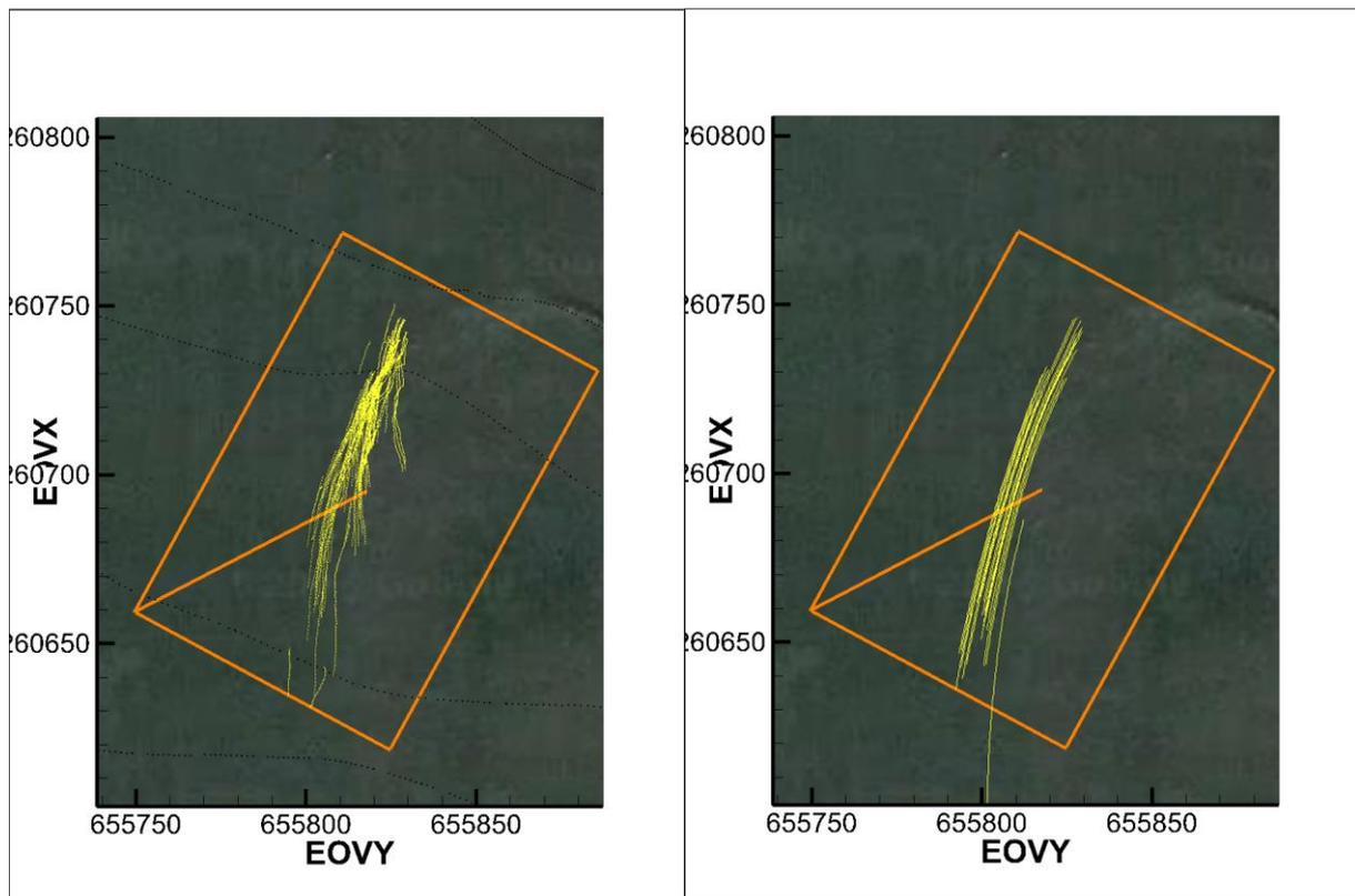
**Figure 19.** Comparison of trajectories calculated from PTV (left) and ADCP (right) measurements
