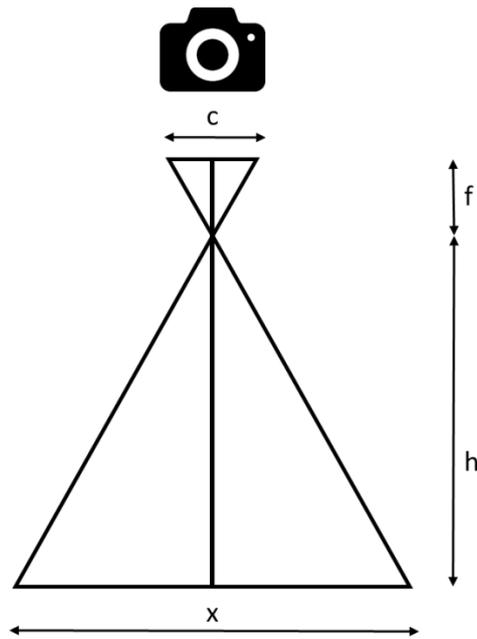
**Figure 15.** Size of image recorded from UAV
