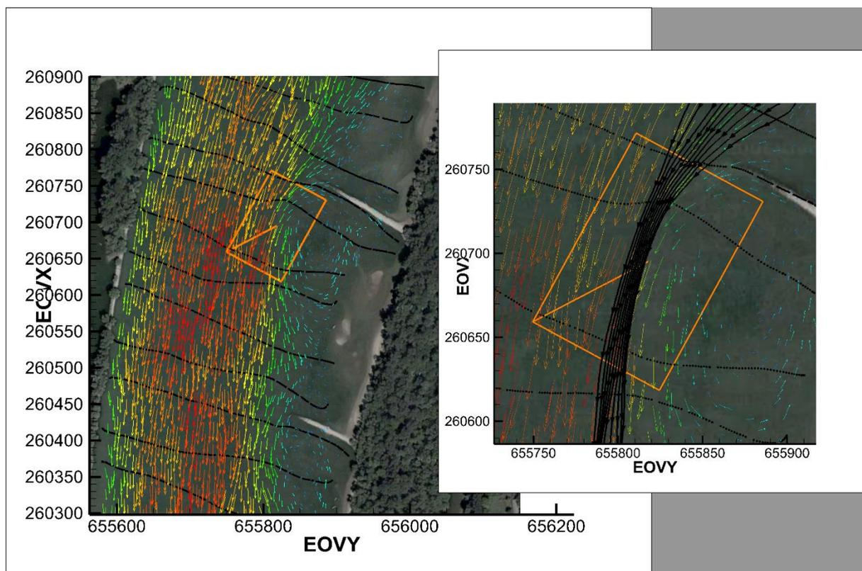
**Figure 18.** Spatially averaged velocity distribution from the ADCP measurements
