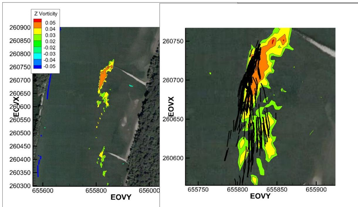
**Figure 22.** Calculated vorticity field from ADCP measurements and tracer trajectories from PTV.
