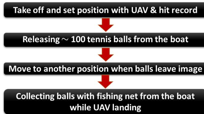
*Figure 4. Steps of UAV measurement*
