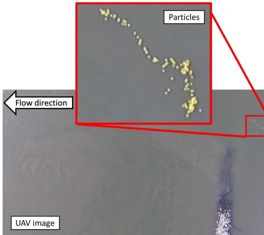
*Figure 6. Tennis balls almost reaching the groyne, after releasing them from the boat*
