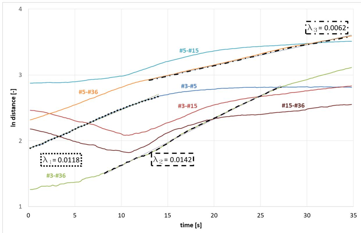
**Figure 23.** Distance of particles #3, #5, #15, #36 from each other with the Lyapunov exponents
